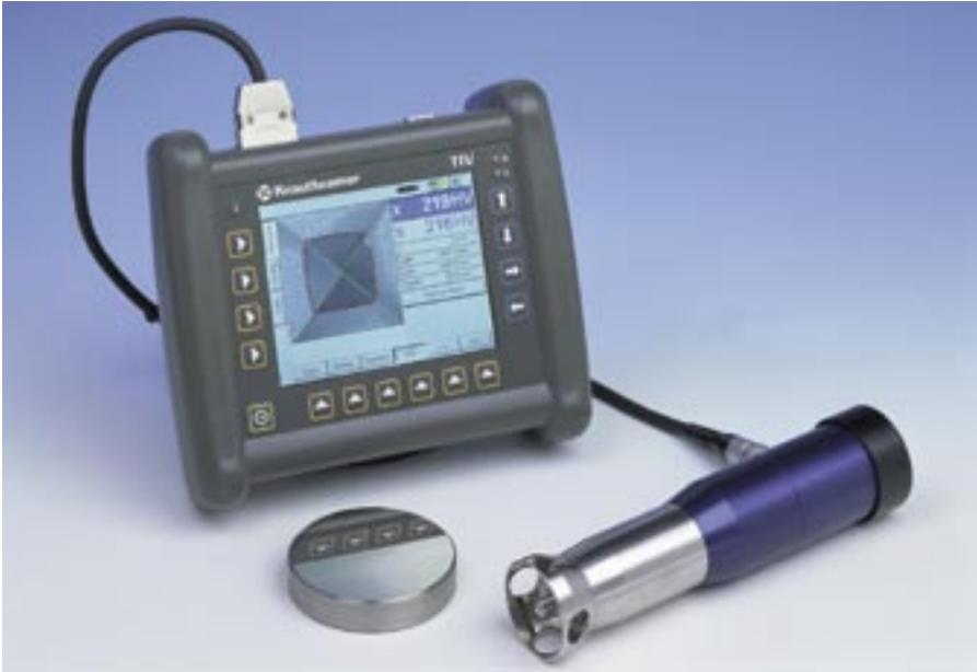
The TIV hardness tester with probe and hardness reference block. The probe contains high-tech features – the optical system and the CCD camera enable viewing through the diamond. Direction independance is also a proof of the patented GE technology: you can measure in any direction – without any additional settings.
